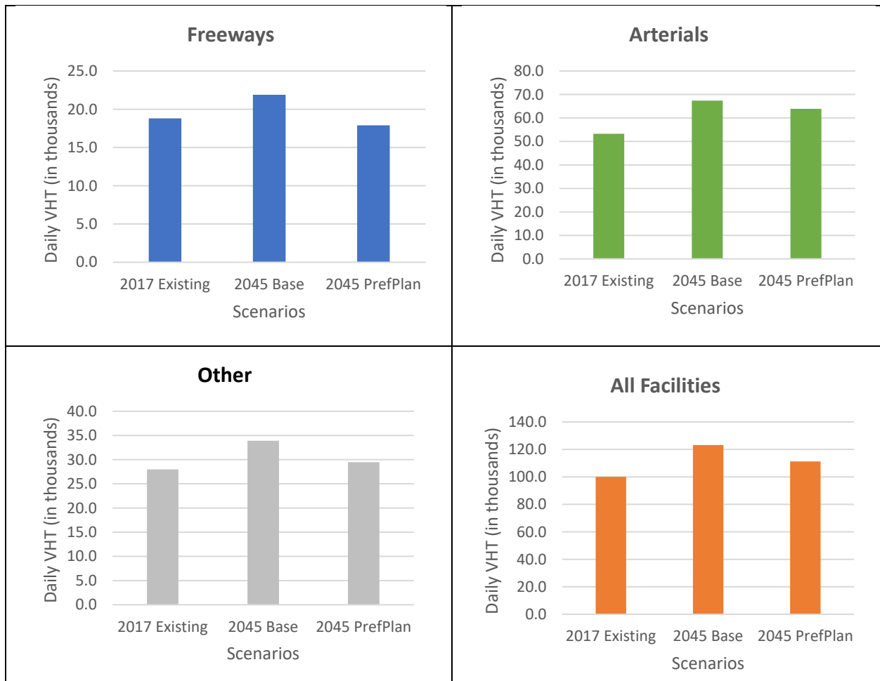
Figure 15: Daily VHT by Facility Type within the Palmdale Sphere of Influence for All Scenarios
